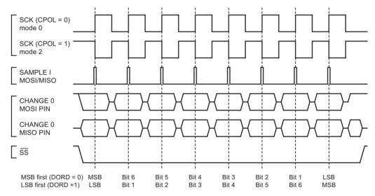
Figure 15-4. SPI Transfer Format with CPHA = 1
