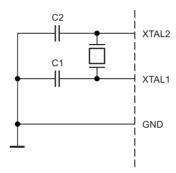
The Oscillator can operate in three different modes, each optimized for a specific frequency range. The operating mode is selected by the fuses CKSEL3..1 as shown in Table 5-3.
