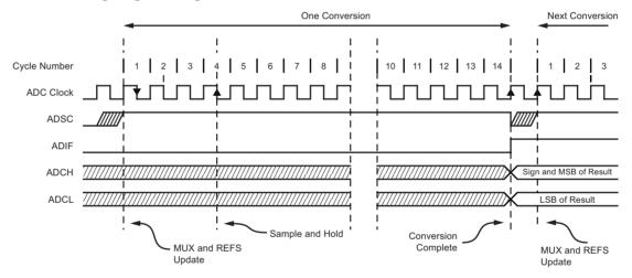
Figure 18-6. ADC Timing Diagram, Auto Triggered Conversion
