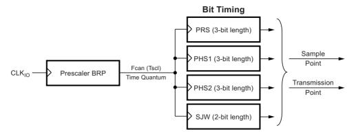
Figure 16-8. General Structure of a Bit Period
