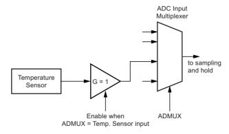
The measured voltage has a linear relationship to the temperature as described in Table 18-3. The voltage sensitivity is approximately  $2.5 \text{mV}/^{\circ}\text{C}$  and the accuracy of the temperature measurement is  $\pm 10^{\circ}\text{C}$  after bandgap calibration.
