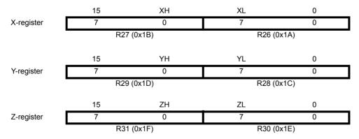
In the different addressing modes these address registers have functions as fixed displacement, automatic increment, and automatic decrement (see the instruction set reference for details).
