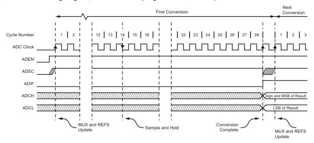
Figure 18-5. ADC Timing Diagram, Single Conversion
