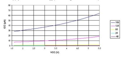
Figure 27-10. Power-down Supply Current versus V<sub>CC</sub> (Watchdog Timer Enabled)
