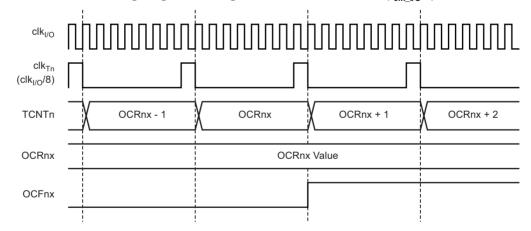
Figure 13-12 shows the count sequence close to TOP in various modes. When using phase and frequency correct PWM mode the OCRnx register is updated at BOTTOM. The timing diagrams will be the same, but TOP should be replaced by BOTTOM, TOP-1 by BOTTOM+1 and so on. The same renaming applies for modes that set the TOVn Flag at BOTTOM.
