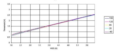
Figure 27-23. Reset Input Threshold Voltage versus V<sub>CC</sub> (VIL, Reset Pin Read As '0')
