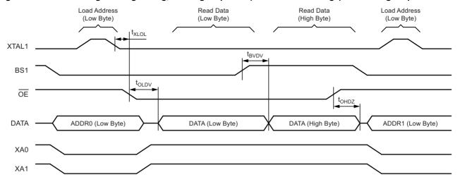
Note: 1. The timing requirements shown in Figure 25-7 on page 268 (i.e., t<sub>DVXH</sub>, t<sub>XHXL</sub>, and t<sub>XLDX</sub>) also apply to reading operation.
