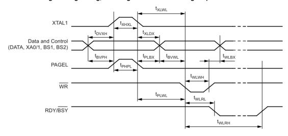
Figure 26-6. Parallel Programming Timing, Loading Sequence with Timing Requirements<sup>(1)</sup>
