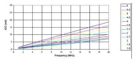
Figure 27-7. IIdle Supply Current versus V<sub>CC</sub> (Internal RC Oscillator, 8MHz)
