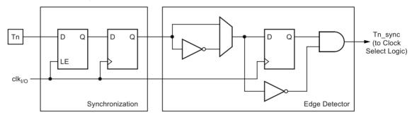
The synchronization and edge detector logic introduces a delay of 2.5 to 3.5 system clock cycles from an edge has been applied to the Tn/T0 pin to the counter is updated.
