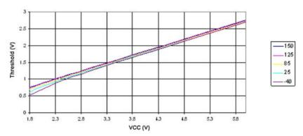
Figure 27-21. I/O Pin Input Hysteresis Voltage versus  $V_{CC}$
