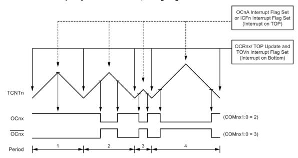
The Timer/Counter overflow flag (TOVn) is set at the same timer clock cycle as the OCRnx registers are updated with the double buffer value (at BOTTOM). When either OCRnA or ICRn is used for defining the TOP value, the OCnA or ICFn flag is set when TCNTn has reached TOP. The interrupt flags can then be used to generate an interrupt each time the counter reaches the TOP or BOTTOM value.
