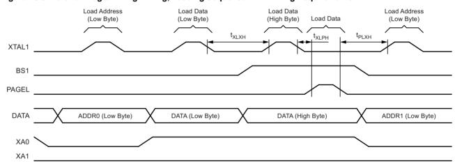
Note: 1. The timing requirements shown in Figure 25-7 on page 268 (i.e., t<sub>DVXH</sub>, t<sub>XHXL</sub>, and t<sub>XLDX</sub>) also apply to loading operation.
