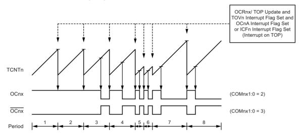
The Timer/Counter overflow flag (TOVn) is set each time the counter reaches TOP. In addition the OCnA or ICFn Flag is set at the same timer clock cycle as TOVn is set when either OCRnA or ICRn is used for defining the TOP value. If one of the interrupts are enabled, the interrupt handler routine can be used for updating the TOP and compare values.
