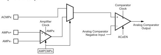
The amplifier clock comes from the ADC and is equal to the ADC Clock divided by 8.
