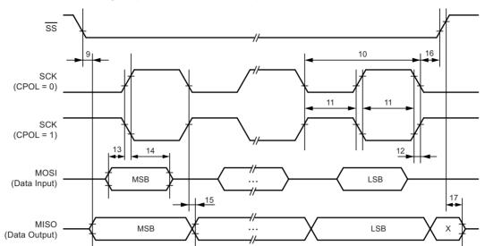
Figure 26-4. SPI Interface Timing Requirements (Slave Mode)
