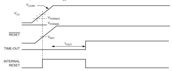
Figure 7-3. MCU Start-up, RESET Extended Externally
