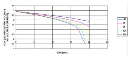
Figure 27-17. I/O Pin Low Output Voltage versus Source Current (V<sub>CC</sub> = 5V)
