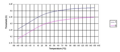
Figure 27-27. BOD Thresholds versus Temperature (BODLEVEL Is 2.7V)
