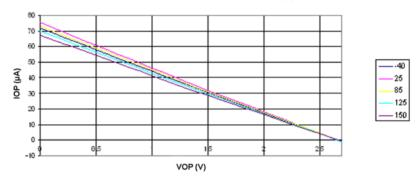
Figure 27-13. Reset Pull-up Resistor Current versus Reset Pin Voltage (V<sub>CC</sub> = 5V)
