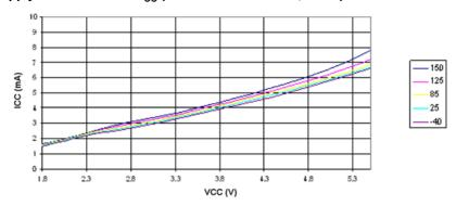
Figure 27-4. Active Supply Current versus V<sub>CC</sub> (Internal PLL Oscillator, 16MHz)
