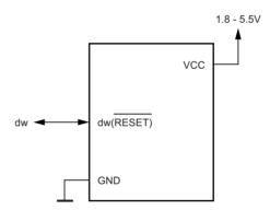
Figure 23-1 shows the schematic of a target MCU, with debugWIRE enabled, and the emulator connector. The system clock is not affected by debugWIRE and will always be the clock source selected by the CKSEL Fuses.
