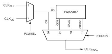
PCLKSELn bit in PSC control register (PCTL) is used to select the clock source.
