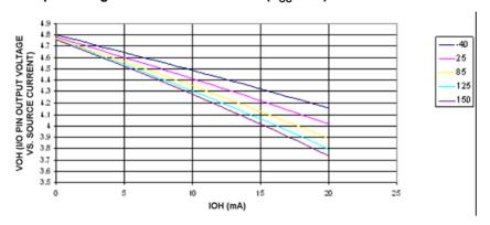
Figure 27-16. I/O Pin Output Voltage versus Source Current (V<sub>CC</sub> = 3V)
