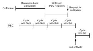
The software can stop the cycle before the end to update the values and restart a new PSC cycle.
