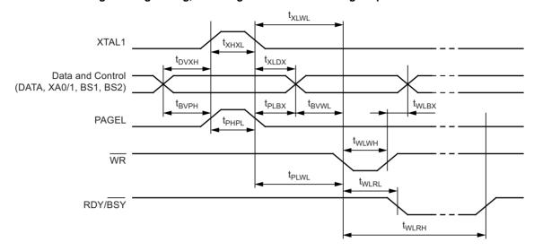
Figure 25-8. Parallel Programming Timing, Loading Sequence with Timing Requirements<sup>(1)</sup>
