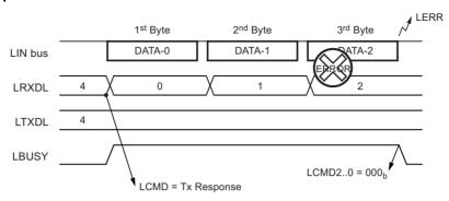
Note: Information on response (ex: error on byte) is only available at the end of the serialization/de-serialization of the byte.
