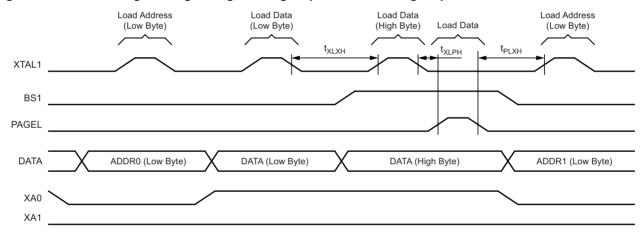
Note: 1. The timing requirements shown in Figure 25-7 (i.e.,  $t_{DVXH}$ ,  $t_{XHXL}$ , and  $t_{XLDX}$ ) also apply to loading operation.
