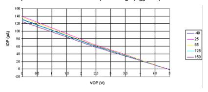
Figure 27-12. I/O Pin Pull-up Resistor Current versus Input Voltage ( $V_{CC} = 2.7V$ )
