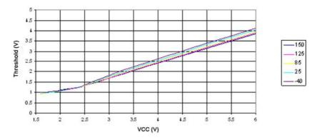
Figure 27-25. XTAL1 Input Threshold Voltage versus V<sub>CC</sub> (XTAL1 Pin Read As '0')
