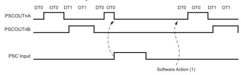
Note: Software action is the setting of the PRUNn bit in PCTLn register.
