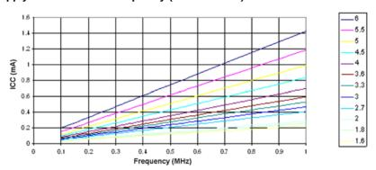
Figure 27-2. Active Supply Current versus Frequency (1 to 24MHz)
