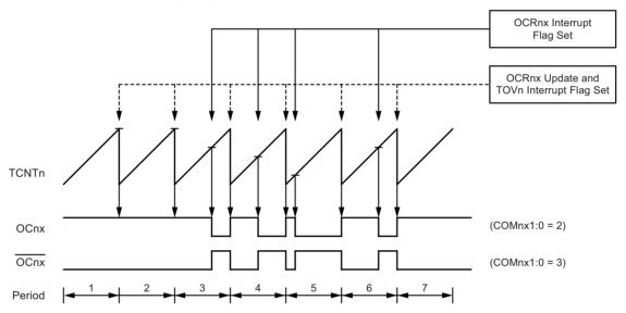
The Timer/Counter overflow flag (TOV0) is set each time the counter reaches TOP. If the interrupt is enabled, the interrupt handler routine can be used for updating the compare value.
