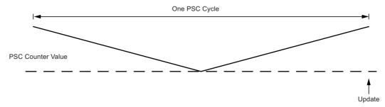
Figure 14-2 on page 118 and Figure 14-3 graphically illustrate the values held in the PSC counter. Centered Mode is like one ramp mode which counts down and then up.
