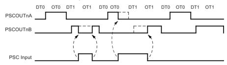
Figure 14-13. PSC Behavior versus PSCn Input A or Input B in Fault Mode 4
