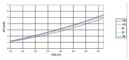
Figure 27-8. Idle Supply Current versus  $V_{CC}$  (Internal PLL Oscillator, 16MHz)
