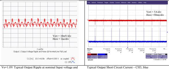
Vo=1.8V Typical Output Ripple at nominal Input voltage and full load at Ta=25 degrees
