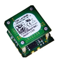
iCG Series DC/DC Power Modules 4.5-14V Input, 6A Output Surface Mount Power Module
