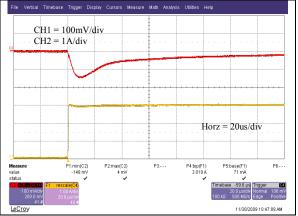
Vo=1.8V Typical output voltage transient response to load step from 25% to 75% of full load with output current slew rate of 10A/uS. (Cext = 1x100uF ceramic capacitor)
