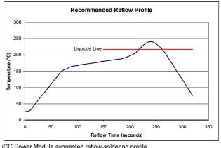
iCG Power Module suggested reflow-soldering profile
