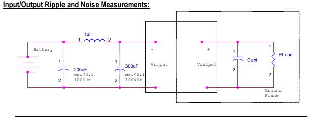
The input reflected ripple is measured with a current probe and oscilloscope. The ripple current is the current through the 1uH inductor.
