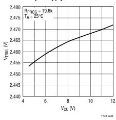
Program Pin Voltage vs Input Supply
