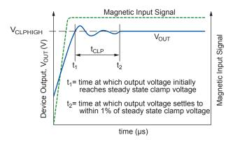
Figure 2. Definition of Delay to Clamp, t<sub>CLP</sub>
