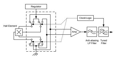
Figure 6. Chopper Stabilization Technique
