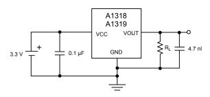
Figure 5. Typical Application Circuit
