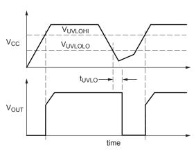
Figure 3. Definition of Undervoltage Lockout
