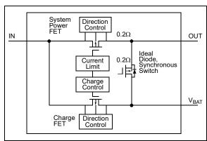
FIGURE 4-2: System Load Sharing Diagram.
