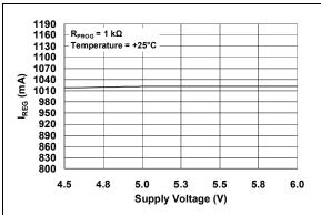
**FIGURE 2-8:** Charge Current (I<sub>OUT</sub>) vs. Supply Voltage (V<sub>DD</sub>).
