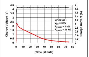
FIGURE 2-28: Complete Charge Cycle (1000 mAh Li-Ion Battery).
