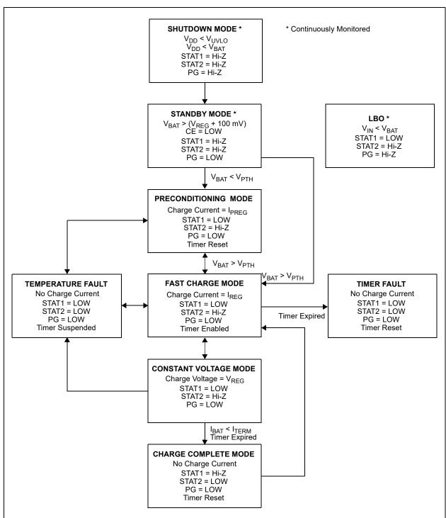
FIGURE 4-1: MCP73871 Device Flow Chart.
