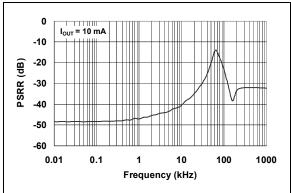
**FIGURE 2-19:** Power Supply Ripple Rejection (PSRR).
