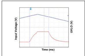
FIGURE 2-24: Undervoltage Lockout.
