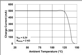
**FIGURE 2-15:** Charge Current  $(I_{OUT})$  vs. Junction Temperature  $(T_J)$ .
