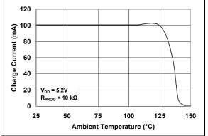
**FIGURE 2-16:** Charge Current  $(I_{OUT})$  vs. Junction Temperature  $(T_J)$ .
